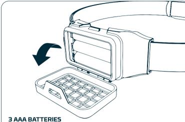
Open the battery compartment, remove old batteries and dispose of properly. Insert 3 new AAA batteries, making sure the negative ( - ) end of the battery faces the spring.
