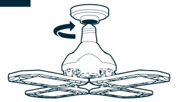
Simply screw the High Bright 9000 into any standard 60w or greater, non-recessed light bulb socket.
