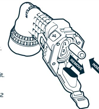
Before operation, move the battery from Compartment 2 to Compartment 1.
